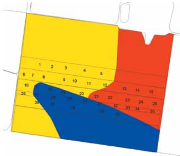
FIGURE 1 Sampling plan: yellow zone = sandy, red zone = loam, blue zone = clay. (Lines across the paddock indicate the boundaries of the fertiliser treatment strips and the numbers represent the pre-designated sampling points.)
