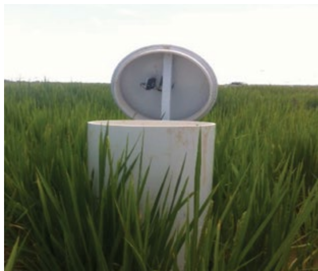
FIGURE 1 Specialised chamber for sampling greenhouse gases in rice
