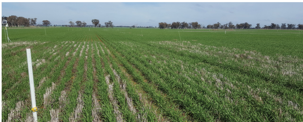
FIGURE 1A The Yarrawonga Victoria site on 27 July 2017, showing yellow 50mm and 300mm Tinytag temperature loggers attached to the PVC tube (left foreground) and weather station (back left)
