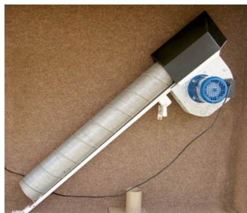
Photo 5: When ordering aeration kits for cone bottom silos, look for one that is simple to install and easy to clean. (Source: Chris Warrick, Primary Business)
