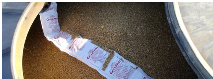
Photo 5: Phosphine in bag chains removes the risk of residue being spilt, but at least 1% of residue will not evolve until it comes into contact with moisture so a respirator and PPE are also required to remove it from the silo. (Source: Chris Warrick, Primary Business)
