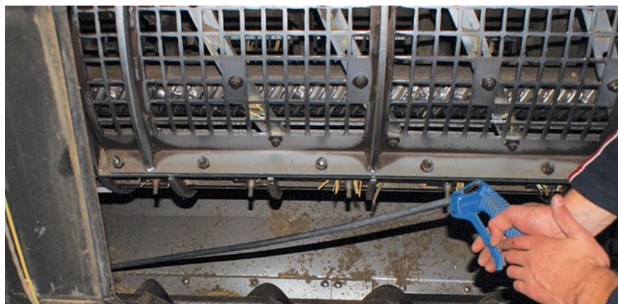
Photo 1: Clean out harvesters and grain handling equipment thoroughly with pressurised air. (Source: Chris Warrick, Primary Business)
